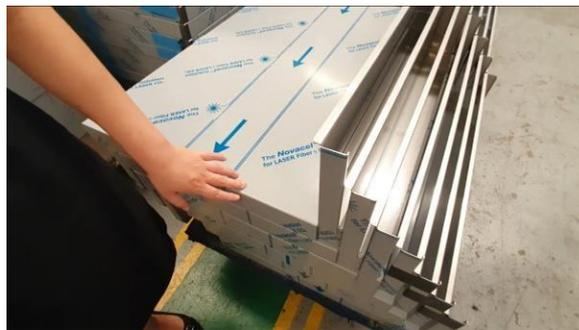
**Gambar 4.i** Proses *bending*.
